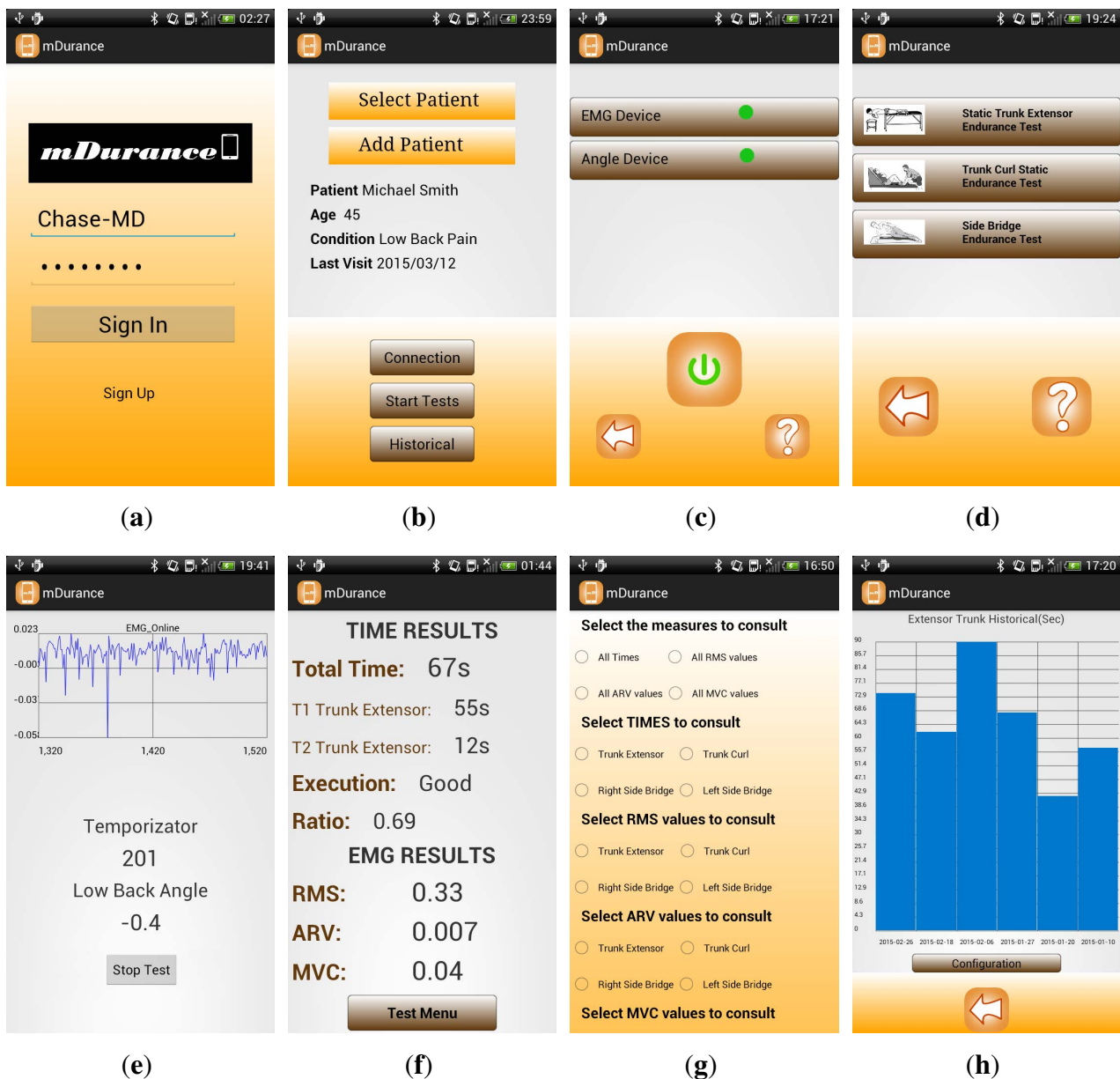
Figure 4. mDurance application snapshots: (a) login; (b) patient selection; (c) sensor connection; (d) endurance test selection; (e) test execution; (f) test results summary; (g) selection of historical attributes to be represented (part of); and (h) historical representation.
