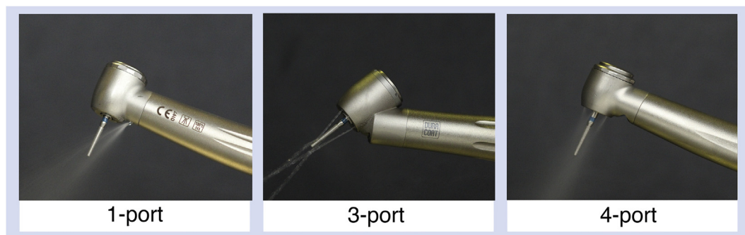
Fig. 1. Water coolant coming out of the 3 different handpieces used in the current study.
