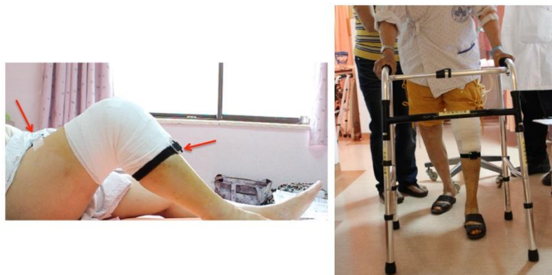
Figure 5. Two sensors were mounted on the anterior side of the thigh and shank.
