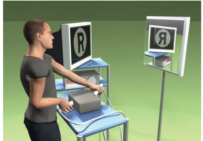
Figure 1. Schematic setting in mirroring the arthroscopic image with a conventional mirror. In this setting, the test subject had no direct view of the original image. Distance with and without the mirror was kept constant.
