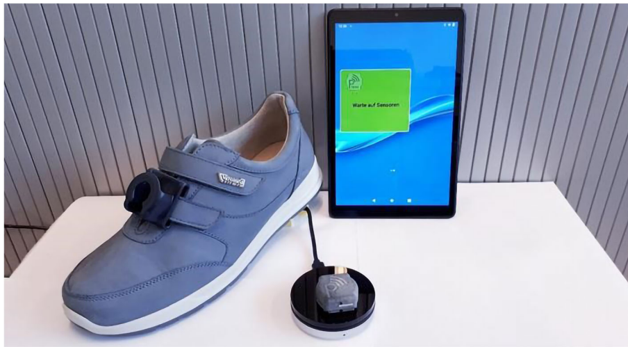
Fig. 3 Technology for activity tracking: tablet-computer, sensor with wireless charger and sensor clip for attachment to shoe
