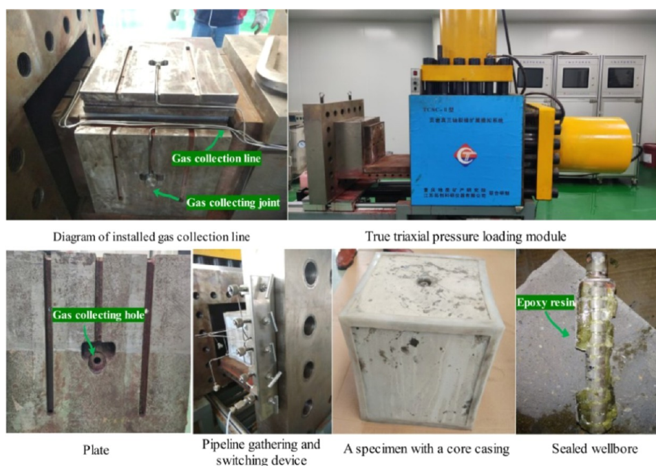
Figure 1. True triaxial stress loading and permeability testing integrated module.
