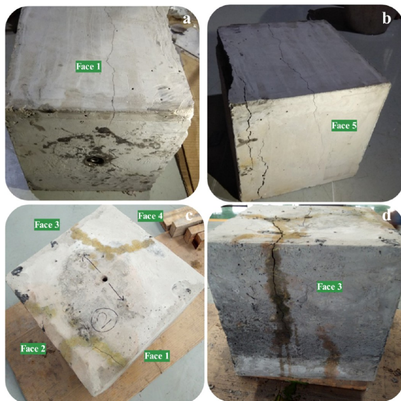
Figure 8. Hydraulic fracturing fracture propagation: (a) Front view of sample 1#, (b) side view of sample 1#, (c) top view of sample 2#, and (d) side view of sample 2#.
