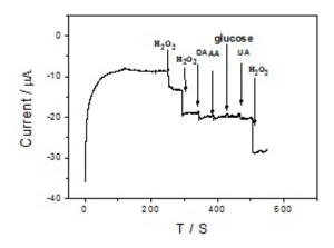
**Figure 8.** Amperometric curves of branch-trunk Ag hierarchical nanostructures/GCE for successive additions of  $H_2O_2$  and different interfering substances in the 0.1 M PBS solution (pH 7.4). The applied potential is -0.5 V.
