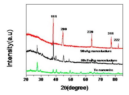
Figure 2. XRD patterns of branch-trunk Ag hierarchical nanostructures generated at different reaction time.
