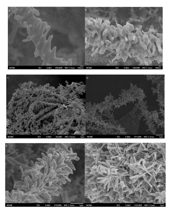
**Figure 1.** Typical SEM images of the branch-trunk Ag hierarchical nanostructures of different reaction time. (**A**,**B**) 30 s ; (**C**,**D**) 60 s; (**E**,**F**) 90 s.
