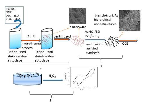
**Figure 3.** Schematic illustration of the formation mechanism of branch-trunk Ag hierarchical nanostructures and branch-trunk Ag hierarchical nanostructure-modified GCE used for detecting H<sub>2</sub>O<sub>2</sub>.
