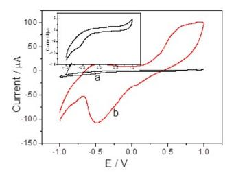
**Figure 4.** CVs of bare electrode (a) and branch-trunk Ag hierarchical nanostructures/GCE (b) in 0.1 M PBS (pH = 7.4) in the presence of 0.5 mM  $H_2O_2$ . Scan rate: 50 mVs<sup>-1</sup>.
