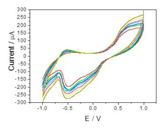
**Figure 5.** CVs of branch-trunk Ag hierarchical nanostructures/GCE in 0.1 M PBS (pH = 7.4) containing, 2 mM, 3 mM, 4 mM, 5 mM, 6 mM, 7 mM, 8 mM  $H_2O_2$ . Scan rate: 50 mVs<sup>-1</sup>.
