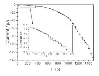
**Figure 6.** Amperometric response of the sensor for successive addition of  $H_2O_2$  in  $N_2$ -saturated 0.1 M PBS (pH = 7.4) solution. The applied potential is -0.5 V, (inset: a partial magnification of the current response toward a low concentration of  $H_2O_2$  solution).
