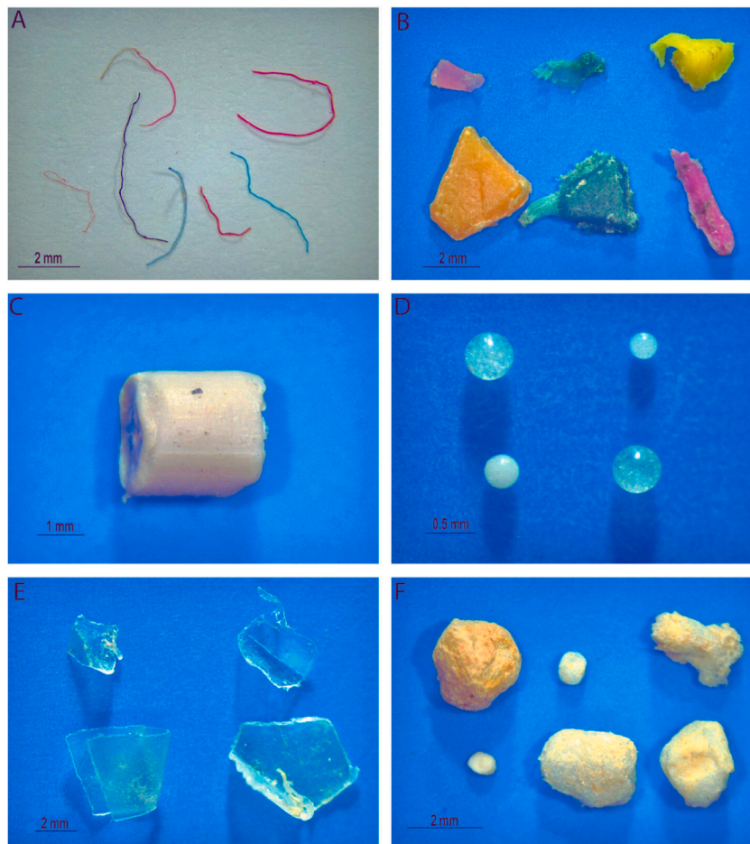
Fig. 3. Representative microplastic particles from the following categories: A) Fibers, B) Fragments, C) Pellets, D) Microbeads, E) Films, and F) Styrofoam found in the Tietê River, São Paulo, Brazil.
