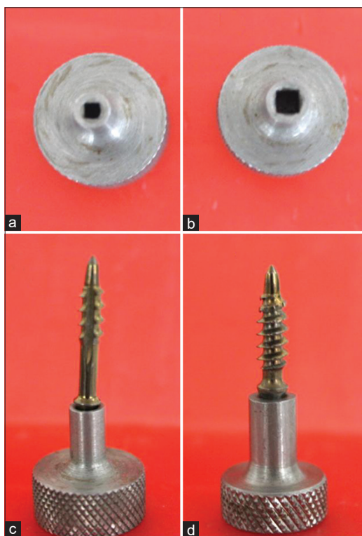
Figure 5: Finger keys for carrying dental implant to the osteotomy site (a and c) narrow head (b and d) wider head
