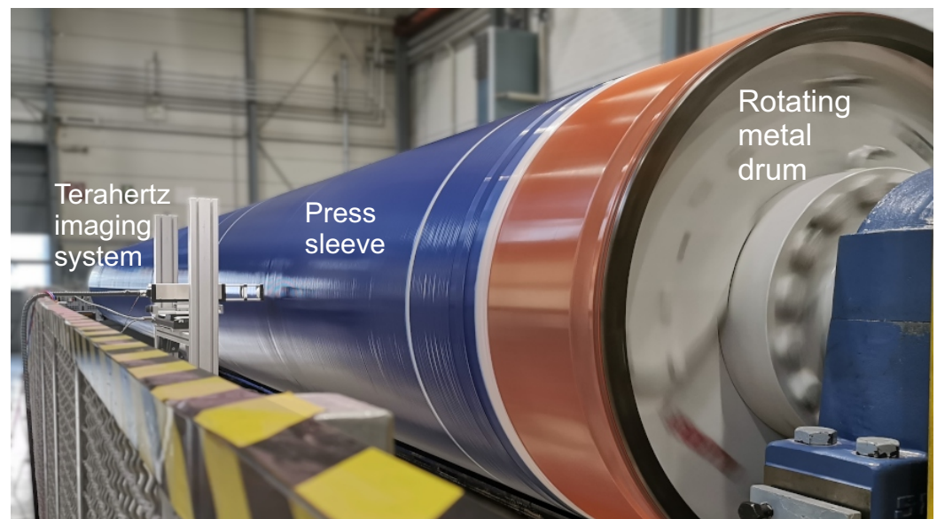
Figure 5. The terahertz imaging system setup in a realistic production environment of press sleeves for the paper industry. The sleeves are investigated within the usual production process to detect possible invisible defects at an early stage of the production line. An area of around 1 square meter of sleeve surface was recorded in this study, limited only by the total travel range of the linear translational axis. Due to the high rotational velocities of up to 150 rpm and large sleeve diameters up to 1.3 m, the terahertz FMCW transceivers are operated at very high data acquisition rates of 20 kHz to yield desired image resolutions of around 0.5 mm.
