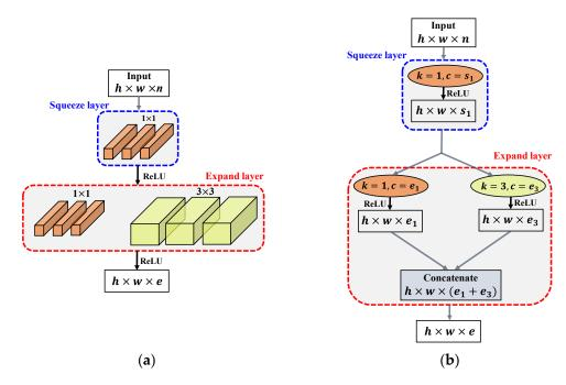
**Figure 1.** Schematic representation of the fire module. (**a**) Fire module structure and (**b**) workflow of the fire module.
