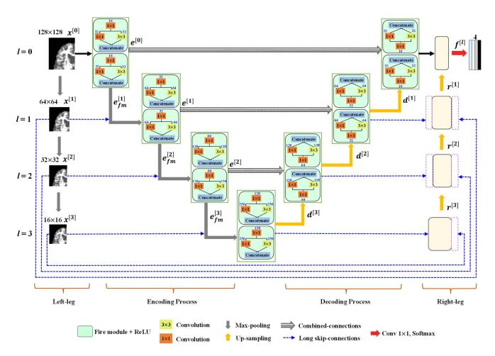
**Figure 3.** The overall architecture of the proposed SM-SegNet model. The fire modules are shown as solid boxes, with the set of feature maps indicated on the top of each box.
