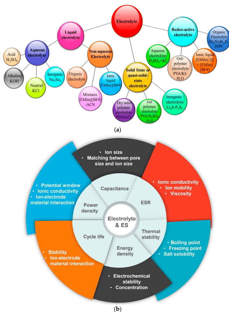
Figure 3. (a) Different types of electrolytes suitable for specific SC applications and (b) impact of the electrolyte on the performance of electrochemical SCs.
