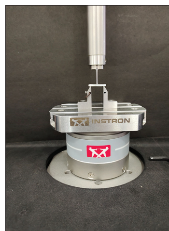
Figure 1: The image depicts the determination of flexural strength using the INSTRON E3000 machine
