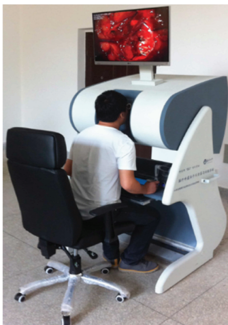
FIGURE 17: The neurosurgery virtual simulation system.
