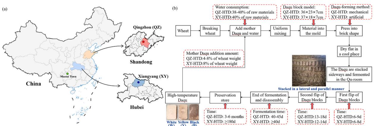
Fig. 1. Distribution map of sampling areas (a) and process flow diagram of Daqu making (b) for high-temperature Daqu (HTD).
