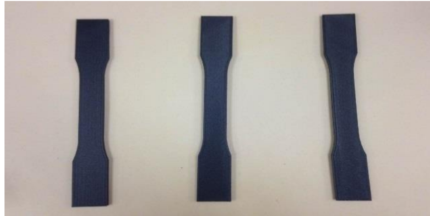
Figure 1. ASTM D 638 Tensile Specimens (6 inches long).
