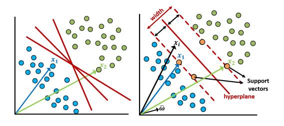
(a) Separating hyper-planes.(b) Best hyper-plane.Figure 4. An overview sketch of Support Vector Machines (SVM) algorithm linear classifier.
