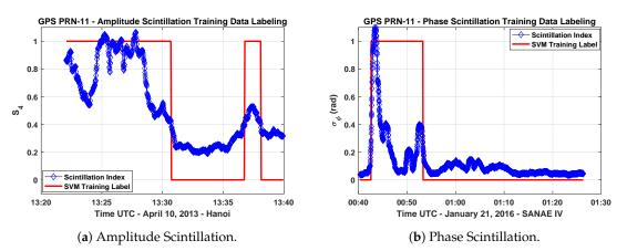
Figure 5. Labeling of the amplitude and phase scintillation index values in the training data sets.
