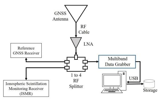
Figure 1. Experimental scintillated GNSS data collection configuration.
