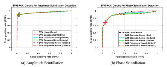
**Figure 7.** Receiver Operating Characteristics (ROC) curves of Support Vector Machines (SVM) methods with different kernel functions.
