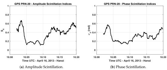
Figure 3. Scintillation index values of GPS L1 C/A PRN-20 signal—16 April 2013 (Hanoi).
