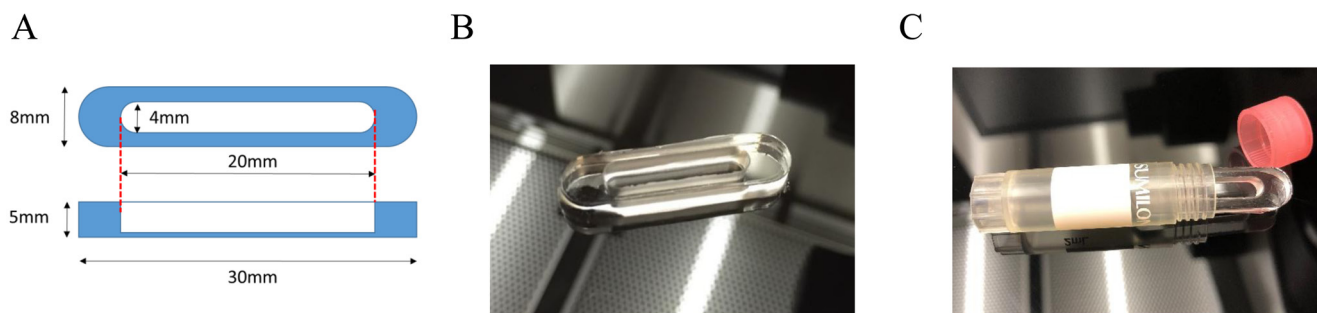
Fig. 1. The new container. (A) The size of the new container was W30 \times D10 \times H5 mm. This size was chosen to allow the easy insertion of the container into a 1.8-ml cryotube. (B) The container (MAYU, STREX) is made of polydimethylsiloxane. The bottom of the container is transparent, which allows the assessment of sperm shape by microscopy. (C) The new container in a 1.8-ml cryotube.
