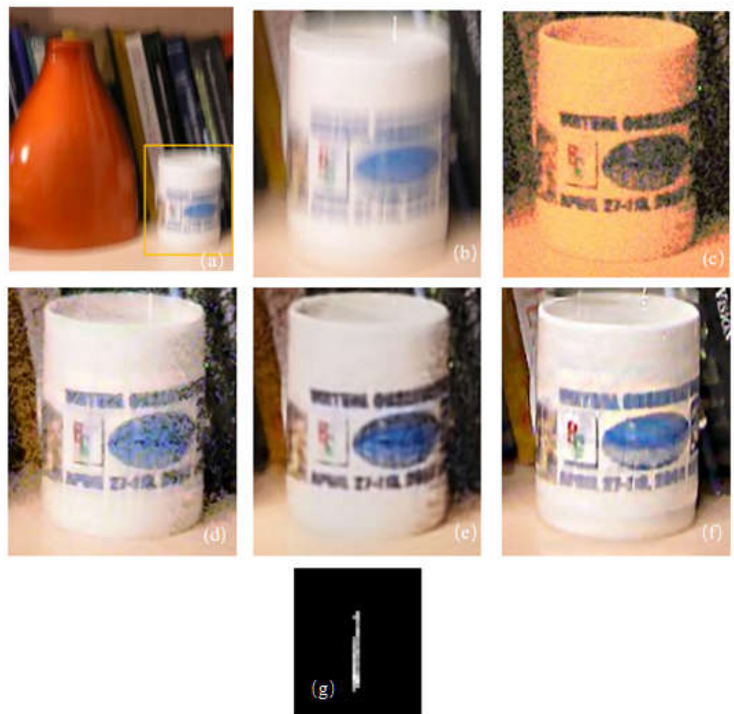
Figure 8. Real image restored experiment; (a) blurred image; (b) blurred image part; (c) Scheme 11. (e) algorithm restored image in [17]; (f) this paper; (g) kernel by proposed.
