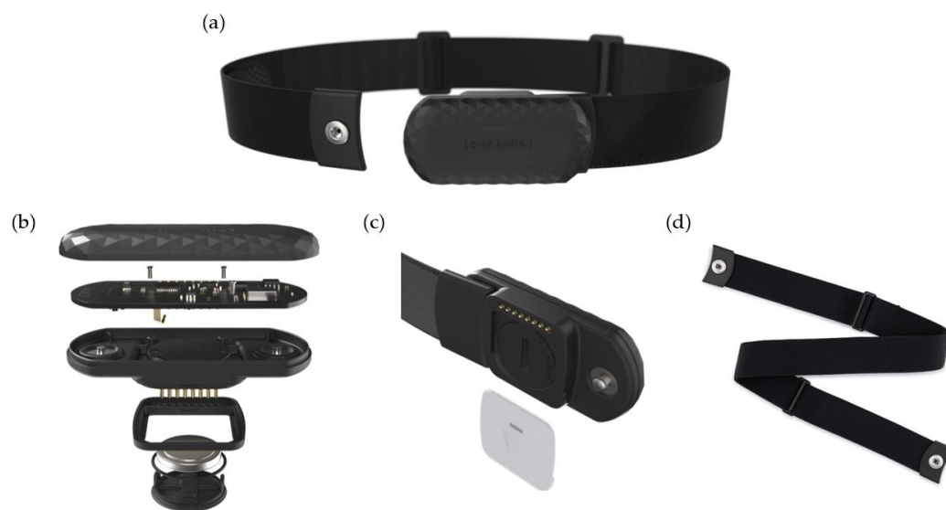
Figure 1. Structure of the wearable device. (a) Complete system, (b) central module (electronics of the system), (c) cartridge, and (d) chest strap.
