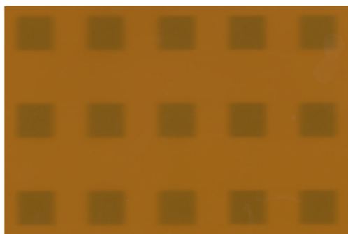
FIGURE 12 Film result of the synchronicity test with the max offset and angular deviation of 0.26 mm and 0.17°
