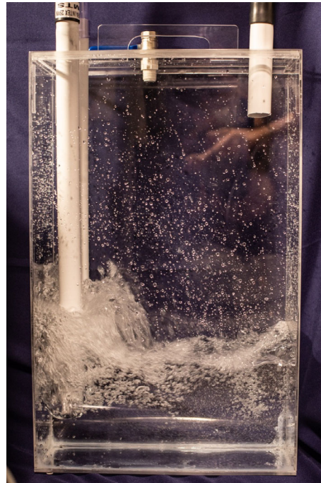
Figure 4 Image of the aspiration and filtering system in operation.
