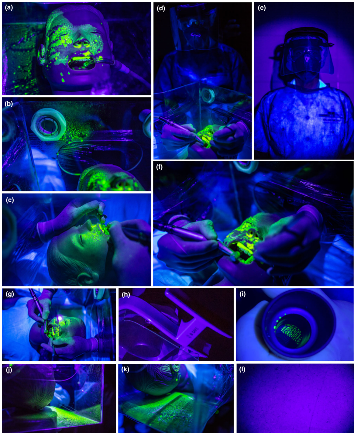
Figure 6 Series of detailed images resulting from the simulation with the device. The fluorescent dye can be observed on the mannequin's face (a, b, c, d, f, g), internal walls of the acrylic chamber (a, b, d, f, g, j, k), internal walls the piping system (i), operator's gloves (c, d, f, g). The dye was not observed in the operator's waist, chest and head regions (e), nor in the light reflector (h) or operating room floor (l).
