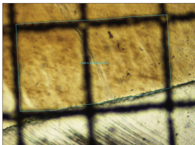
Figure 7b: Photomicrograph of the prepared ground section showing measurement of the area of two rectangular grids on the enamel area (4x)
