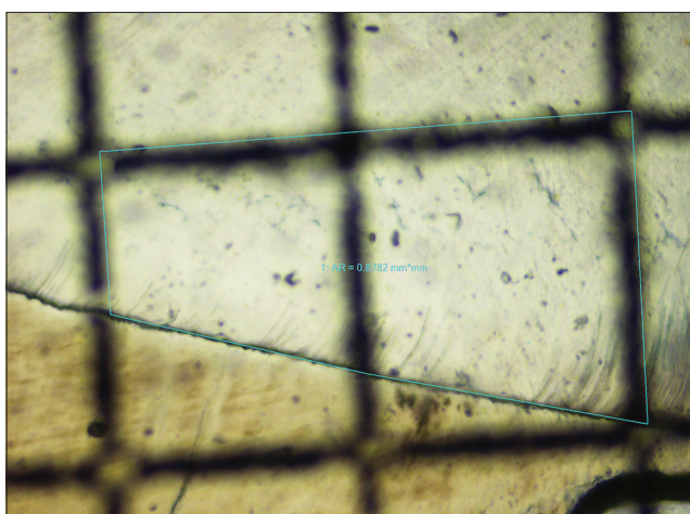
Figure 9b: Photomicrograph of the prepared ground section showing measurement of the area of two rectangular grids on the dentin area (4x)
