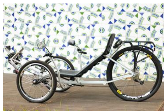
Fig 2. The tadpole trike adapted in this work for mobile FES cycling.
