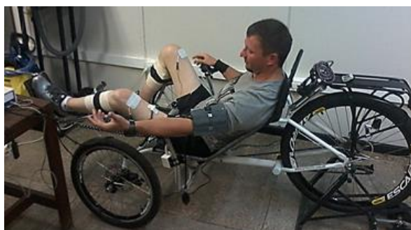
Fig 5. Photograph of stationary set up used during the initial training of the FES-cycling preparation.
