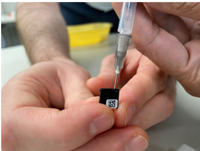
FIGURE 7 Using a 14-gauge needle to inject water within the optically stimulated luminescence dosimeters (OSLDs) to force air out. Compressed air must be used to dry before reading the OSLDs
