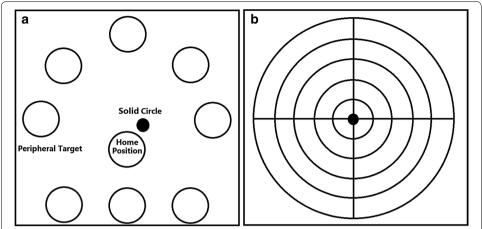
**Fig. 2** The graphical interface of the tasks. **a** The LoS task, with the home position in the middle, the real-time position of the CoP was shown as a solid circle, and 8 targets located around the home position; **b** the interface for finding the home position, the range of movement in the four directions, and the corresponding calibration of the position of the targets
