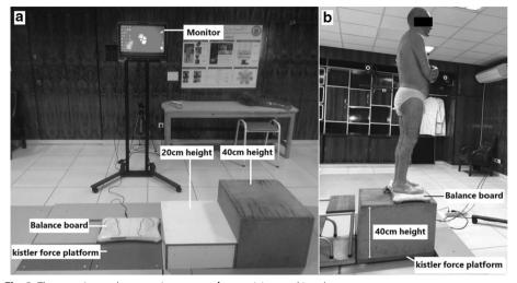
Fig. 3 The experimental setup: a Instrument; b a participant taking the test
