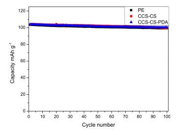
Figure 6. Cycle performance of coin cells with the PE separator, CCS-CS and CCS-CS-PDA.
