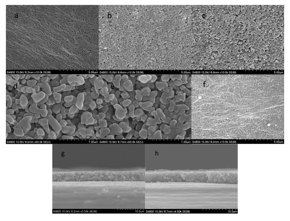
**Figure 1.** SEM morphology: (a) PE, (b,d) CCS-CS, (c,e) CCS-CS-PDA and (f) PE side of CCS-CS-PDA. Cross-section morphology: (g) CCS-CS and (h) CCS-CS-PDA.
