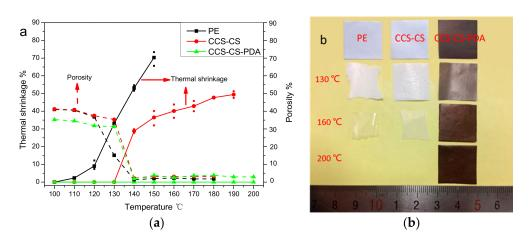
**Figure 2.** (a) Thermal shrinkage and porosity (%) changes of the CCS-CS and CCS-CS-PDA membrane. (b) Photograph of the PE, CCS-CS and CCS-CS-PDA after being held at different temperatures for 30 min.
