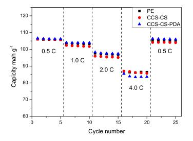
Figure 7. Rate performance of the batteries with the PE separator, CCS-CS and CCS-CS-PDA.
