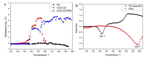
Figure 5. (a) The shutdown behavior of the separator; (b) DSC of the PE separator and PDA.
