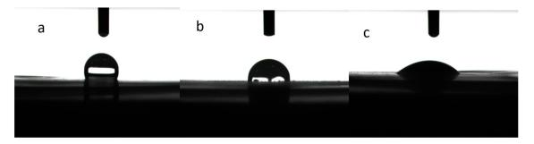
Figure 4. Contact angle tests: (a) PE separator, (b) CCS-CS, (c) CCS-CS-PDA.
