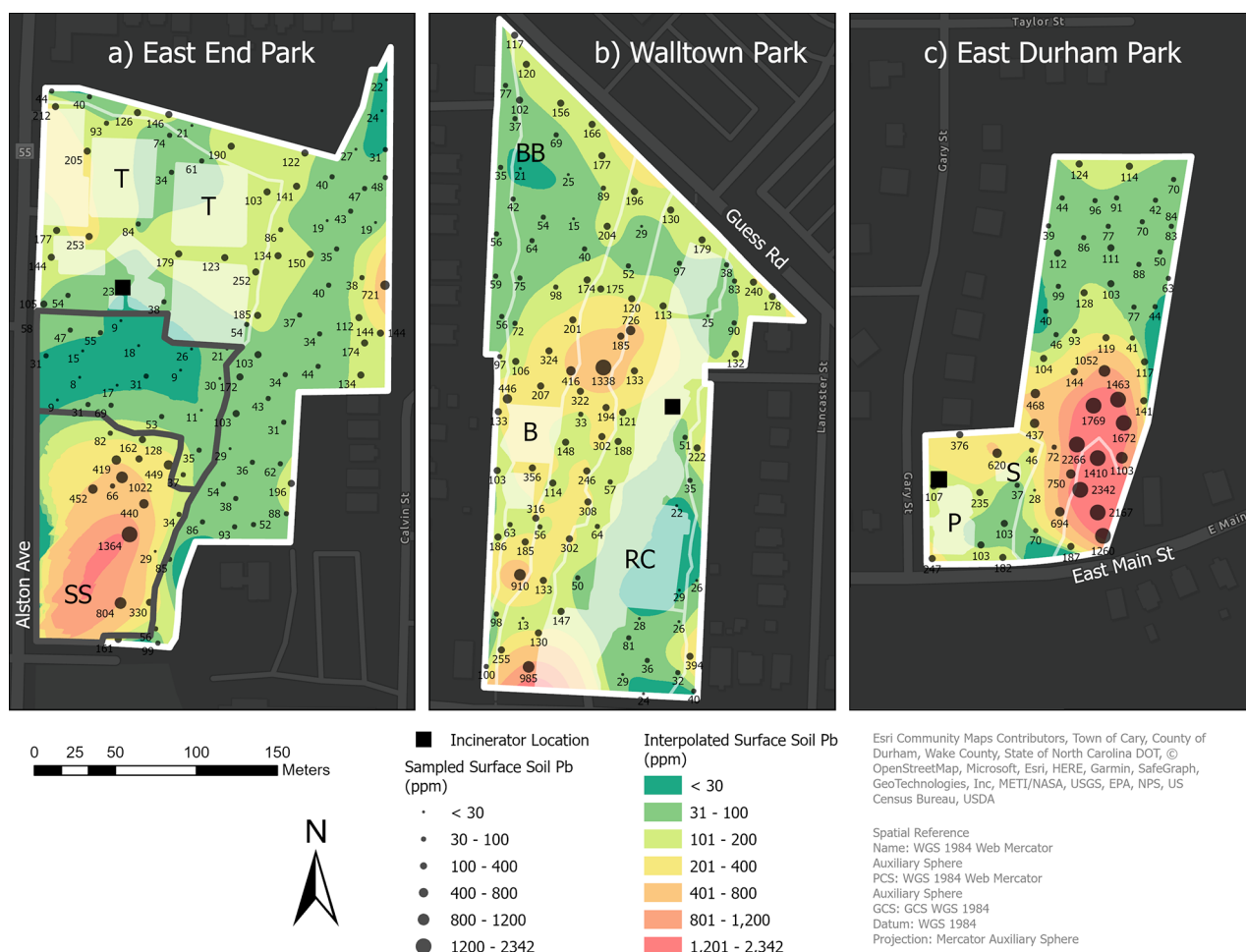
Figure 1. Surface-soil Pb heat maps of (a) East End Park, (b) Walltown Park, and (c) East Durham Park in Durham, North Carolina. In (a) East End Park, “T” marks hard-surface tennis courts, and “SS” is the city’s abandoned Sign and Signal Shop, the latter surrounded by fencing with locked gates indicated by black lines. In (b) Walltown Park, “B”, “BB”, and “RC” are outdoor basketball courts, old baseball field, and community recreation center, respectively. In (c) East Durham Park, “P” and “S” are playgrounds with a jungle gym and picnic shelter, respectively.
