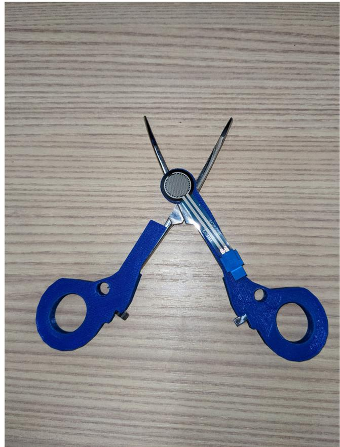
**Figure 1** Final Kelly clamp case prototype with one sensor.
