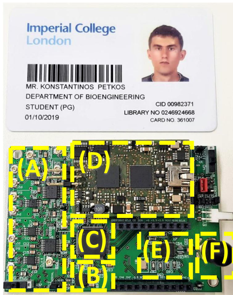
Fig. 4 Structure of the proposed instrument. The instrument's architecture includes: (a) a high-performance, eight-channel (five channels on the main board and another three channels on a stacked PCB that is adjusted on the two headers shown in the picture) AFE, (b) an analog, low-power 3-axis accelerometer, (c) an eight-channel, 24-bit ADC, (d) an FPGA module, (e) a 2 MBps Zigbee transceiver, and (f) a 2.4 GHz antenna
