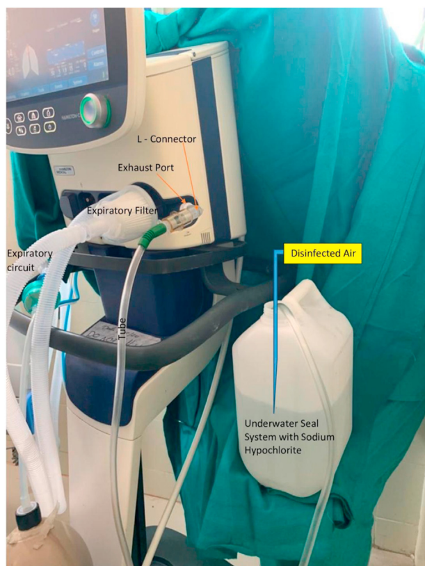
Fig. 1. Ventilator exhaust port with underwater seal assembly.
