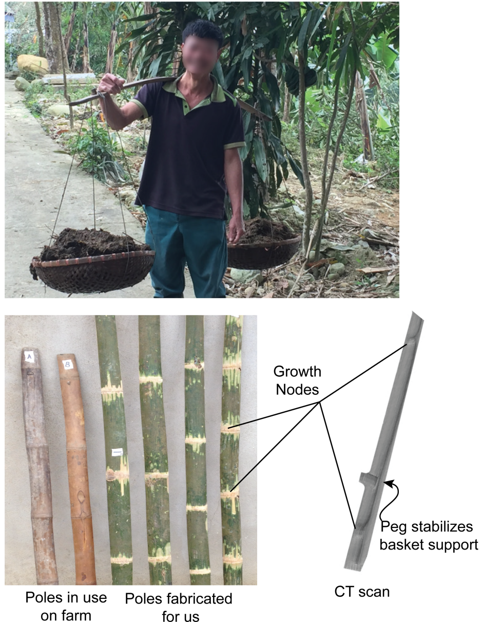
Fig 1. Pole carrying technique and example poles. Top: A farm worker carries a bamboo pole in northern Vietnam. The pole is supported at the shoulder with the hand (same side as the supporting shoulder) resting on top of the forward end to steady the system. Growth nodes are also indicated (Bottom Left: poles used in the study; Bottom Right: CT scan of pole C). These nodes are characterized by a thickening of the cross-section from a portion of a hollow tube to a portion of a solid cylinder.
