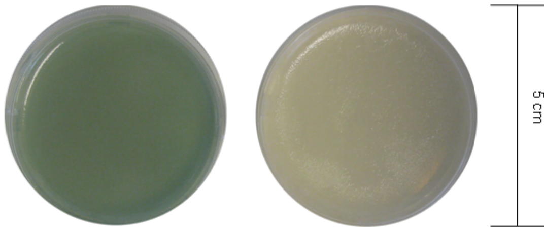
Figure 5: Plasma source B, argon plasma, treatment duration 6 min, Pseudomonas aeruginosa SG81 (left, dense growth) and Staphylococcus epidermidis RP62A (right, dense growth)
