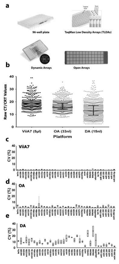
**Figure 1.** Platform overview and co-efficient of variation analysis. (a) Representative pictures of the four platforms. (b) CT/CRT values from all samples. Lines indicate median and IQR. Boxplots (median, 10–90th percentile) of the CV distribution for (c) ViiA7, (d) OA and (e) DA.
