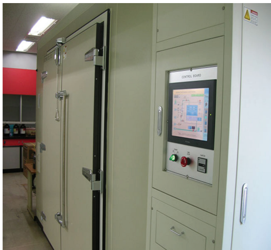
FIGURE 1: Emission test chamber system, 5 m 3 in size (Ecopro, Republic of Korea).
