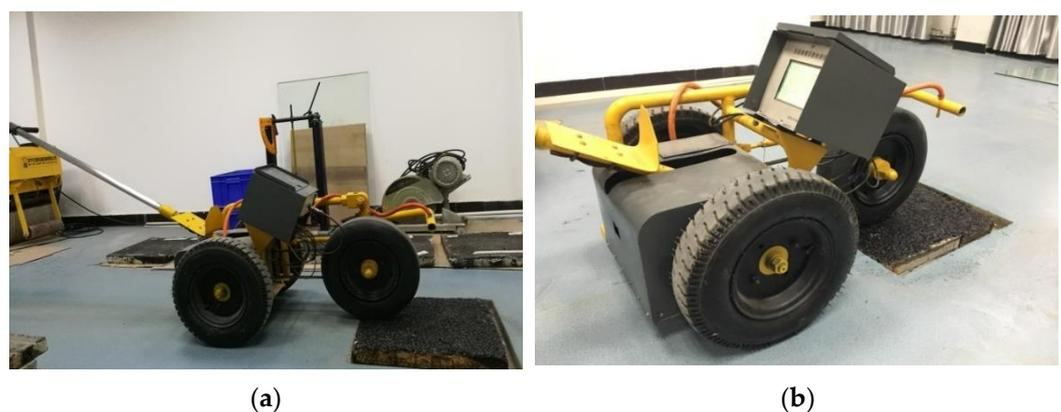
Figure 3. The Walking Friction Tester. (a) Test wheel contact the specimen; (b) Test procedure.
