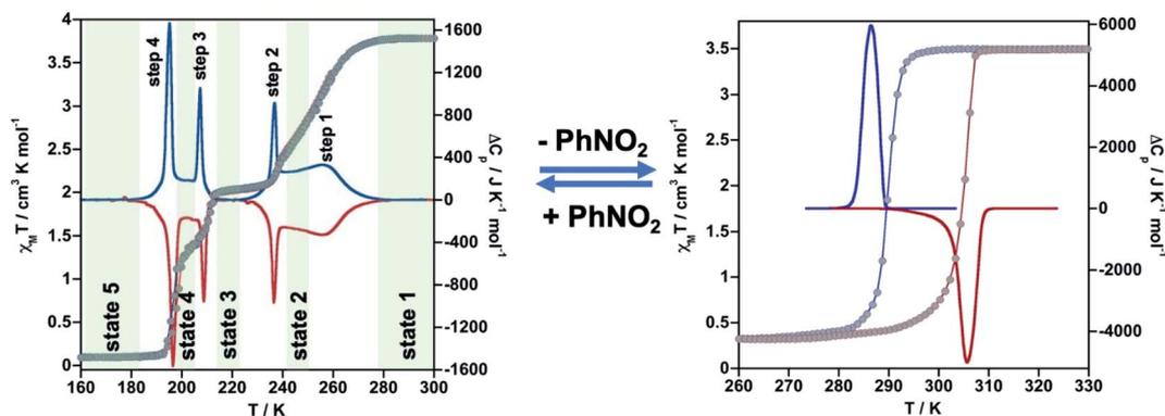
Fig. 1 Thermal dependence of magnetic (grey circles) and calorimetric properties of  $1 \cdot \text{PhNO}_2$  (left) and  $1$  (right). Blue and red curves correspond to the cooling and heating modes in  $\Delta C_p$ .
