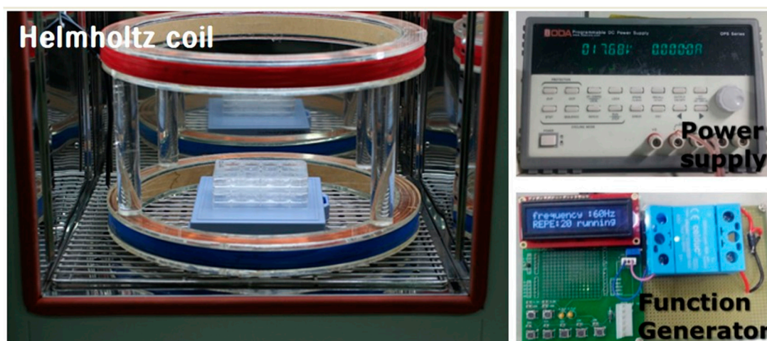
Figure 1. Photograph of the electromagnetic field (EMF) device. Pulsed EMF was generated using a pair of Helmholtz coils of 40 cm diameter and 15 cm separation.
