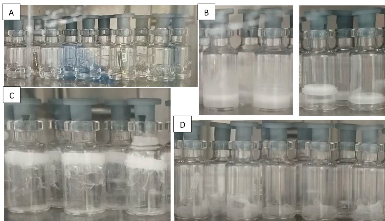
Figure 1. (A) Bubbling observed in untreated vials filled with 5% w/w mannitol + 0.02% w/v Tween 80 (the chamber pressure was 6 mbar). (B) Fogging observed in sulfate-treated vials (left), but not in TopLyo vials (right) filled with 5% w/w mannitol, immediately after nucleation. (C) Blow up observed in TopLyo vials filled with 5% w/w sucrose + 0.02% w/v Tween 80. (D) Irregular product in TopLyo vials filled with demineralized water, caused by boiling. All these pictures were taken immediately after nucleation.
