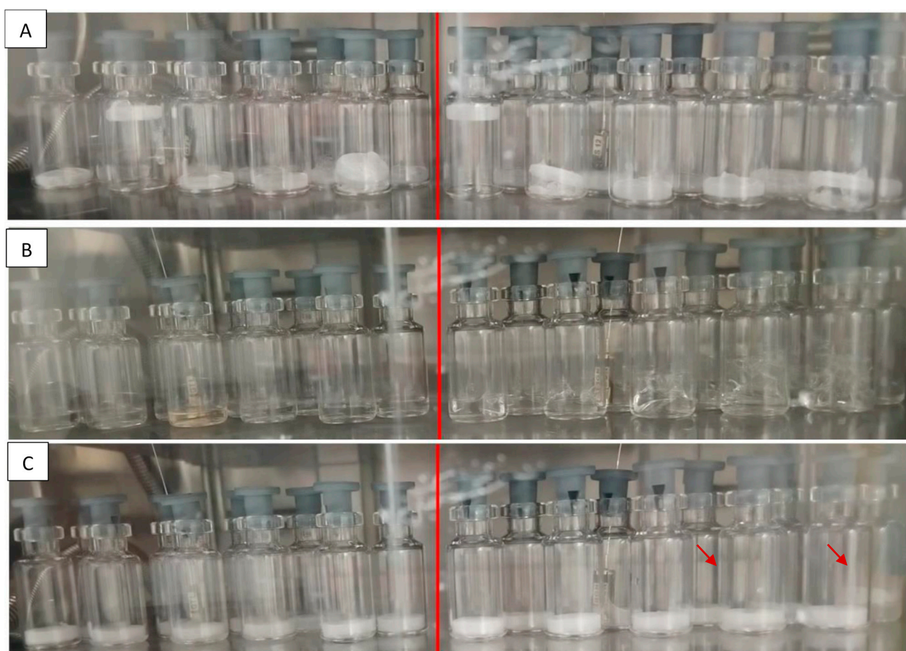
Figure 2. Two groups of TopLyo vials were filled with the DW (A) or DW + TW80 (B,C) formulations. (A) Defects due to boiling were observed in both degassed (left) and non-degassed (right) DW vials. (B) In the non-degassed DW + TW80 group (right), bubbling phenomena were observed while inducing nucleation. (C) The morphology of the DW + TW80 frozen product was acceptable when degassing was performed (left), whereas small defects due to bubbling (as indicated by arrows) could be observed in the non-degassed samples (right). All these pictures were taken immediately after nucleation.
