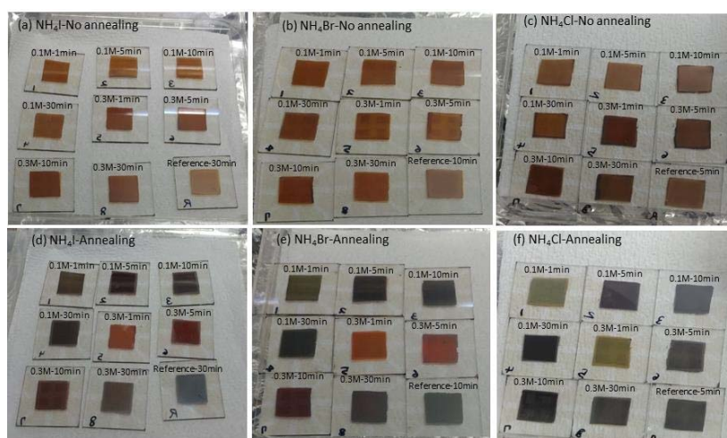
Figure 3. Optical images of \text{CH}_3\text{NH}_3\text{PbI}_{3-x}\text{Cl}_x layers prepared with (a) \text{NH}_4\text{I} , (b) \text{NH}_4\text{Br} , and (c) \text{NH}_4\text{Cl} before annealing process and (d) \text{NH}_4\text{I} , (e) \text{NH}_4\text{Br} , (f) \text{NH}_4\text{Cl} after annealing process. The color change occurred after annealing.
