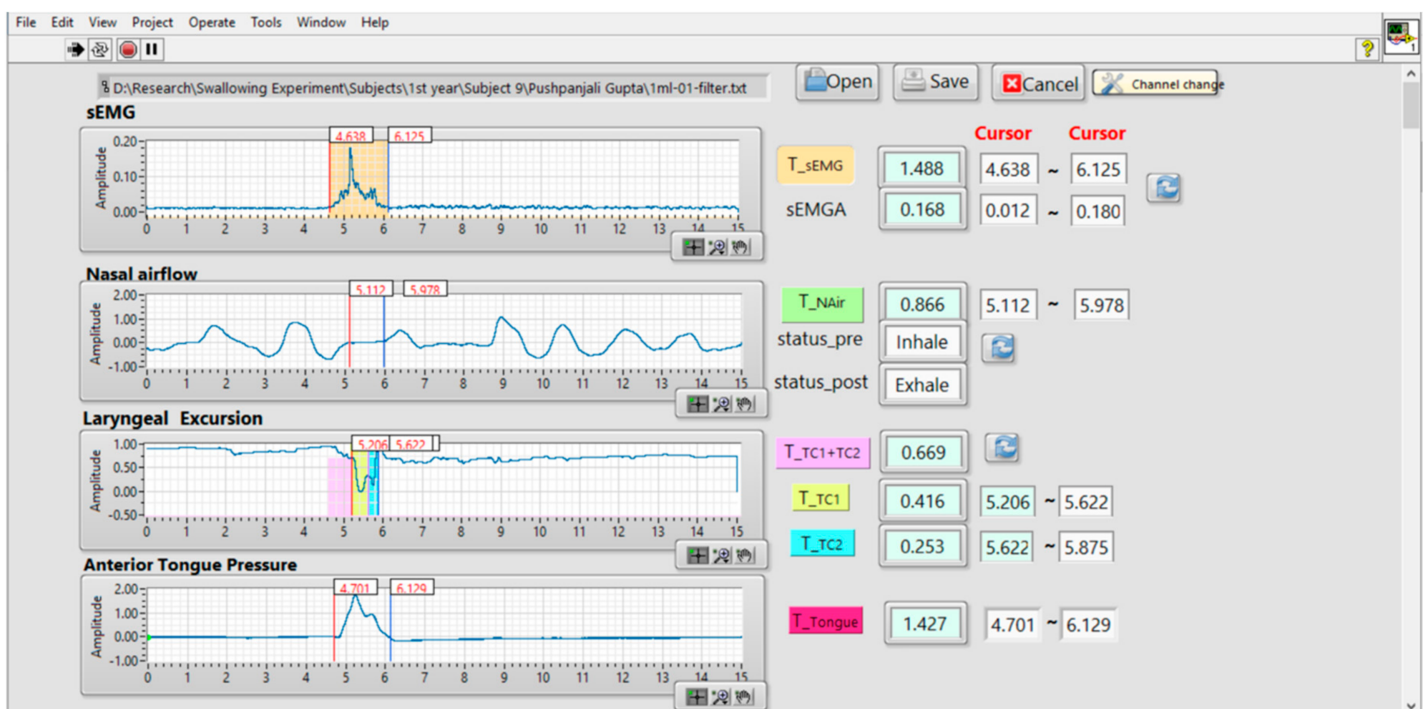
Figure 8. Snapshot of the autodetection program. This program was implemented in LabVIEW [21] language.
