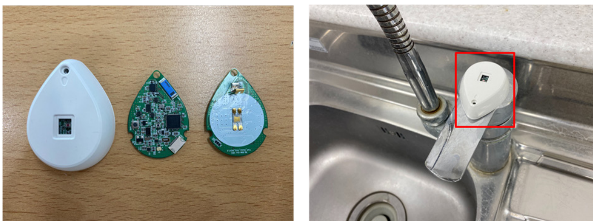
Figure 15. External Sensor Device (Faucet).
