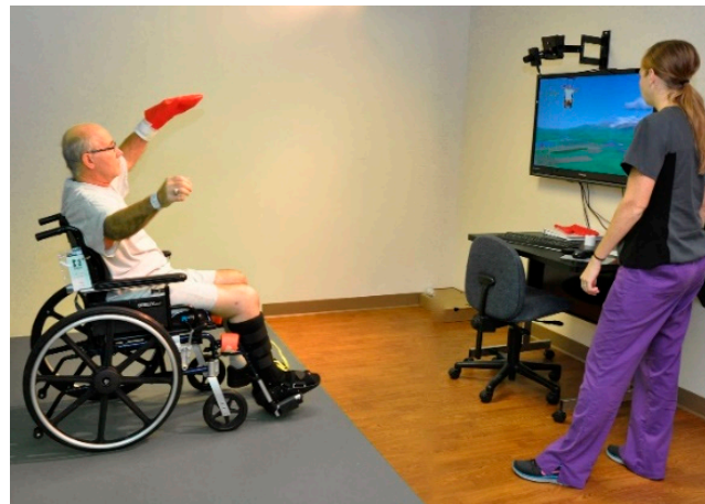
Figure 8. This VR system can track upper- and lower-body movements and features pre-built functions similar to physical therapy exercises. The system enables a physical therapist to select patient-specific motions and games that best match the patient’s needs and goals [83]. Source: GestureTek’s IREX Immersive Rehabilitation Exercise Systems.
