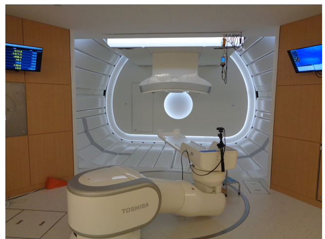
Figure 1. Compact rotating gantry room of our carbon-ion facility.
