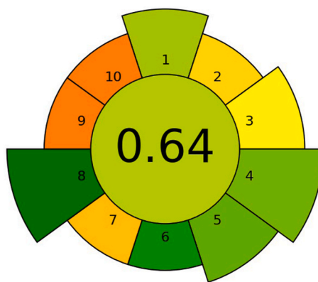
Fig. 7. The AGREEprep pictogram of etrasimod forced degradation study. Legend: AGREEprep: 1 – sampling, 2 – hazardous materials, 3 – sustainability, renewability, and reusability of materials, 4 – waste, 5 – economy of a sample, 6 – sample throughput, 7 – automatization, 8 – energy consumption, 9 – analytical instrumentation, 10 – operator's safety.
