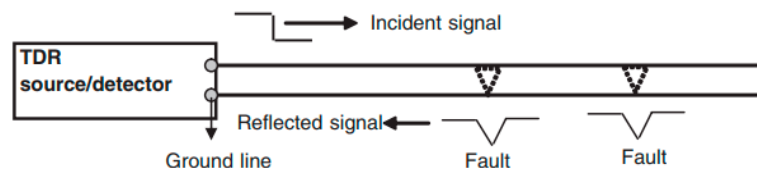
Figure 16. Schematic illustration of TDR defect detection method [115].
