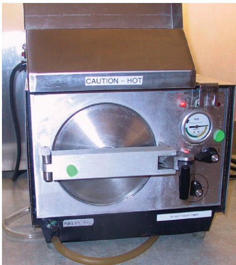
FIG. 6-12 Chemiclave chemical vapor sterilizer. (From Bird DL, Robinson DS: Torres & Ehrlich Modern Dental Assisting , St. Louis, 2009, Saunders/Elsevier.)
