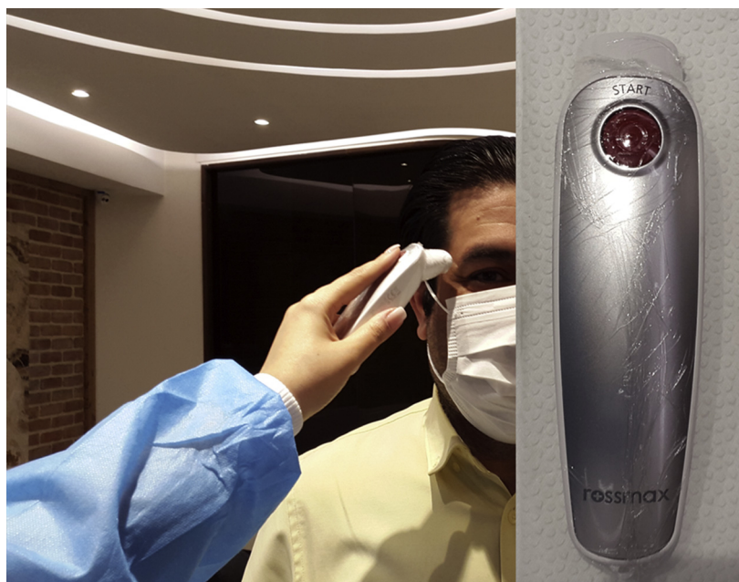
Fig 2. The 1-second measurement no-contact temple thermometer (HA500, Rossmax International Ltd, Taipei, Taiwan) without contacting skin (5 cm distance) is an appropriate choice to measure the body temperature and prevent cross-contamination.
