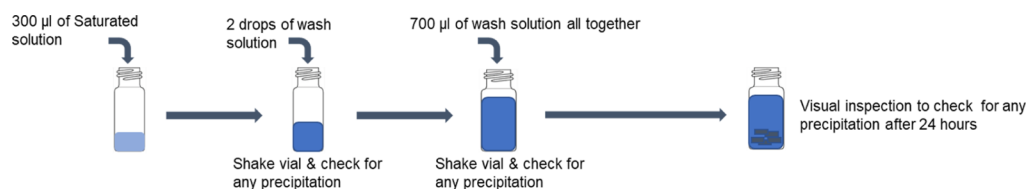
Figure 2. Glass vial precipitation detection method.
