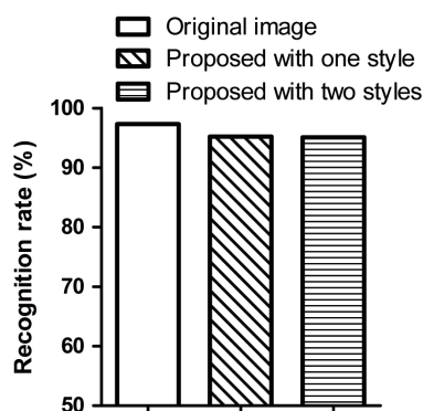
Figure 6. Rates of recognition by DeCAPTCHA. “Proposed” is style-plugged CAPTCHA.
